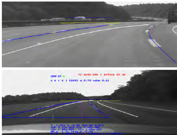
Figure 5: Driving tube (bright overlay) and lane model (dark) while the Ego is driving near the right border of the lane, but still inside the lane
