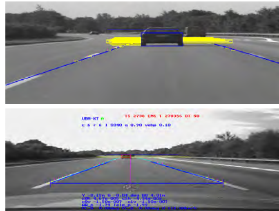
Figure 4: Clipping of search windows using bounding boxes of OVs
