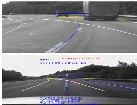
Figure 6: Driving tube and lane model while performing a lane change
