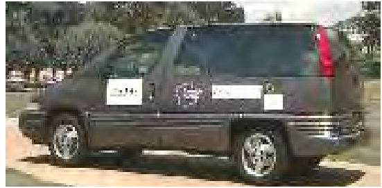
Figure 8: Navlab 5 of CMU, which performed the demo ‘Hands-off through America’ (automatic lateral control by vision over 98 % of the distance) in 1995.
