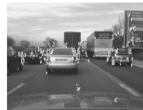
Figure 7: Nonplanarity’ features on first pyramid level of original video-field (cell size m_c = 2 , n_c = 2 , yielding 125 x 370 cells). Mel size = 2·2 cells; even with these parameters, reducing computing time by more than an order of magnitude, the same image regions with stable features for tracking are found (on larger scales only). [Image compressed 2:1 horizontally after feature extraction.].
