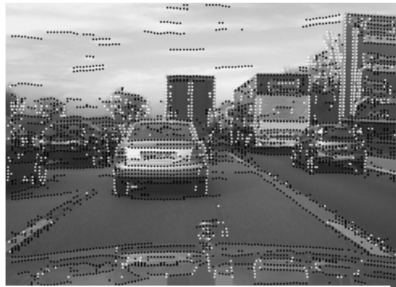
Figure 8: Edges from extreme values in gradient components in row- (white) and column search (black), [m = n = 3, m_c = 2, n_c = 1] .
