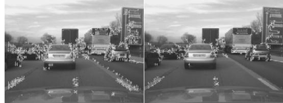
Figure 6: Distribution of ‘nonplanarity’ features in a typical highway scene. Left: threshold ErrMax = 5 %; right: ErrMax = 7.5 %. Results from row- and column-search are super-imposed (horizontal and vertical white line elements); cell size m_c = 2 , n_c = 1 , mel size 3·3.
